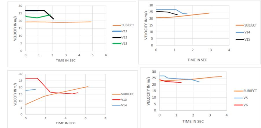
These velocity profiles define how the drivers behaved in 0% and 50% penetration of connected-automated vehicle conditions. The velocity profiles show that when the driver's chose gaps between the automated and connected vehicles, the effect on mainline vehicles was higher, that is, the vehicle had to decelerate much more than when merging between conventional vehicles.
