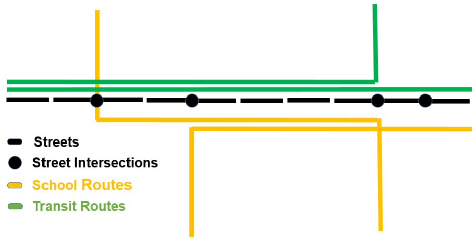
Figure 10: Comparison of school and public transit routes with road reference layer. Due to the overlapping nature of these three layers, it is important that each is split at street intersections.
