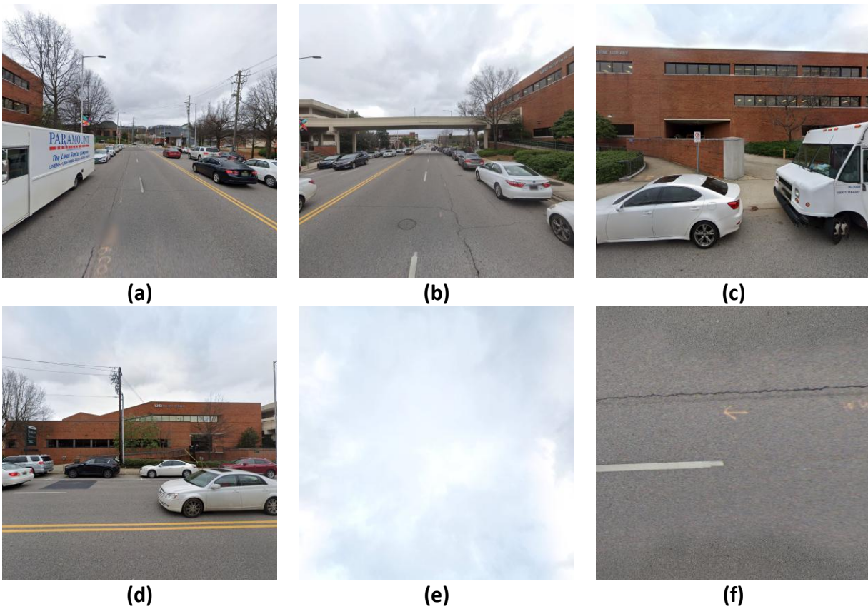
Figure 9. CubeMap output of panoramic image: (a) Back of GSV car, (b) Front of GSV car, (c) Right of GSV car, (d) Left of GSV car, (e) Top of GSV car, (f) Bottom of GSV car.
